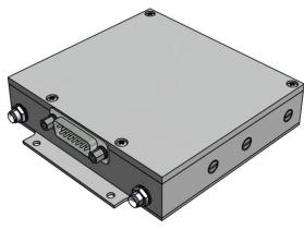
The preselector PS512 is digitally tunable filter operating from 30 MHz to 512 MHz. This module consists of three (3) internal tunable bandpass filters (the frequency range divided between them in the following way: 30-96 MHz, 96-262 MHz and 262-512 MHz). PS512 uses serial or parallel interface for tuning.
