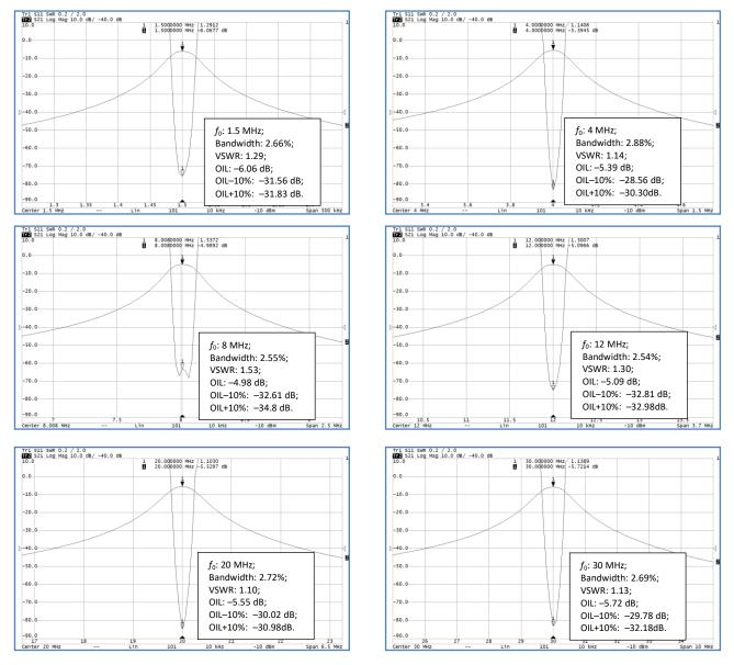
**Note:** $f_0$ — tuning frequency;VSWR — VSWR at  $f_0$  frequency;OIL — insertion loss at  $f_0$ ; OIL-10% — insertion loss at 0,9 $f_0$ ;OIL+10% — insertion loss at 1,1 $f_0$ .
