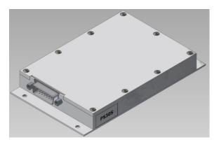
The preselector PS1.5-30S is digitally tunable filter operating from 1.5 MHz to 30 MHz. This module consists of two (2) internal tunable bandpass filters (the frequency range divided between them in the following way: 1.5-6.7 MHz and 6.7-30 MHz) and the internal amplifier (it compensates filter's insertion losses). PS1.5-30S uses serial interface for tuning.
